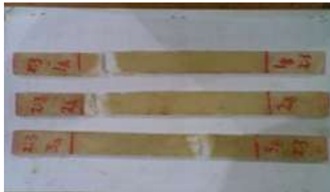
Figure 1 Sample specimen of tensile test result
