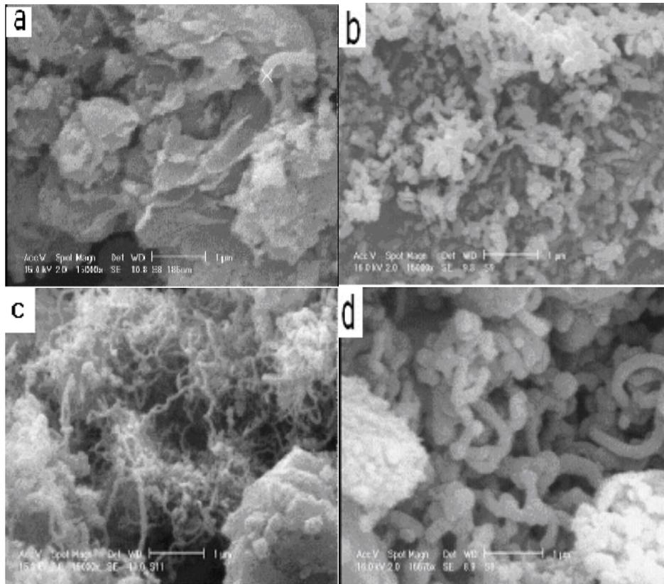
**Fig3. SEM images of synthesized of CNTs on a) Fe nanoparticle without any substrate (compare a and c in which all of the synthesis conditions is same) and other images are related to Fe (nm)/Al<sub>2</sub>O<sub>3</sub> under different growth temperatures b) 875°C c) 925°C and d) 985°C. As can be seen in 875°C CNTs are very short with low yield and in 985°C CNTs are very large diameters. (b and d)**
