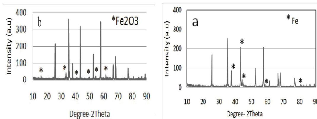
Fig1. XRD patterns of prepared catalyst a) Fe (nm)/Al<sub>2</sub>O<sub>3</sub> and b) Fe<sub>2</sub>O<sub>3</sub>/Al<sub>2</sub>O<sub>3</sub>
