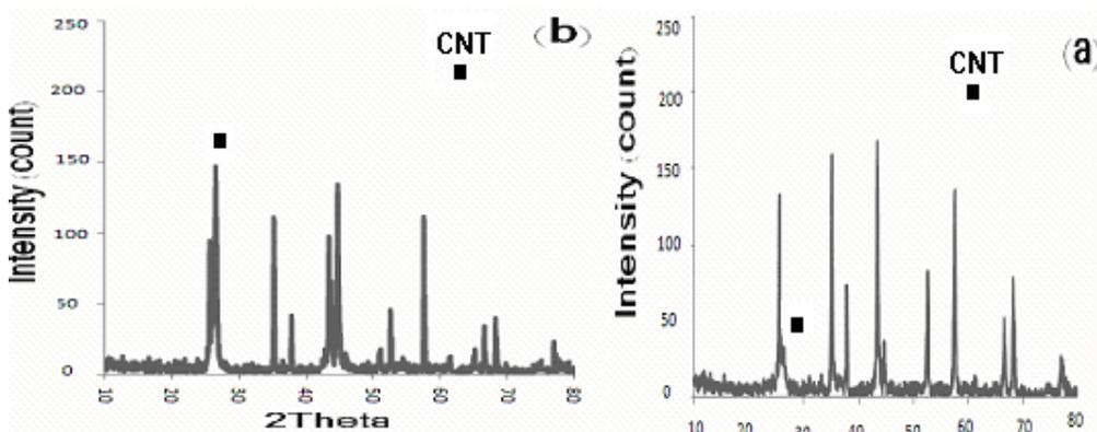
Fig2. XRD patterns of synthesised CNTs on prepared catalytic substrate, a) Fe (nm)/Al<sub>2</sub>O<sub>3</sub>, and b) Fe<sub>2</sub>O<sub>3</sub>/Al<sub>2</sub>O<sub>3</sub> containing 40 % Salt). The peaks corresponding to CNTs are marked in the figure.
