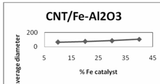
**Fig7. Increasing of CNT 's outer diameter with increasing in concentration of Fe (NO<sub>3</sub>)<sub>3</sub>.9H<sub>2</sub>O**
