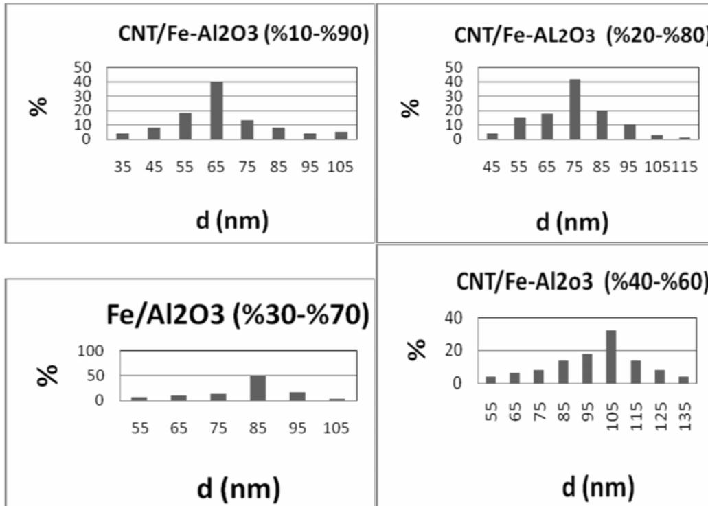
**Fig6. Outside diameter distribution of CNT growth on Fe<sub>2</sub>O<sub>3</sub>/Al<sub>2</sub>O<sub>3</sub> which prepared by second method with different concentration of catalyst. a)10 wt% , b)20 wt% , c)30 wt% and d)40 wt%**
