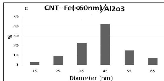
**Fig4. Outside diameter distribution of CNT growth on Fe (nm) / Al<sub>2</sub>O<sub>3</sub> which prepared by first method. (Only one weight percentage of Fe nanoparticles)**
