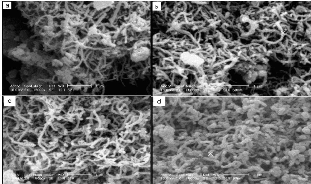
**Fig5. SEM images of the growth of CNTs on  $\text{Fe}_2\text{O}_3/\text{Al}_2\text{O}_3$  with different concentration of salt a) 10 wt%, b) 20 wt% , c)30 wt% and d)40 wt%**
